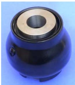
**After a few hours of cleaning, machining and sometimes a small repair on the back, were the clutch lifting lever presses on to the bearing housing, and paint. The clutch thrust bearing assembly is ready for many more miles.**
