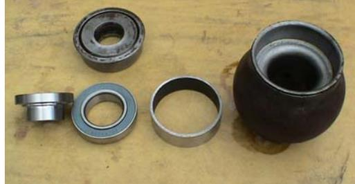
For the bushing in the housing I am using mechanical tubing. It is strong, does not have a seam and it can be easily machined.
