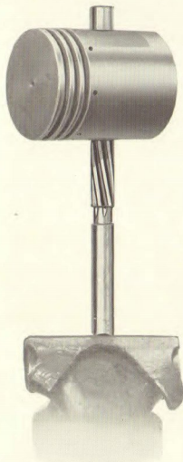
Fig. 35 Align Reaming Piston for Pin Here is shown the proper way to hold the reamer in vise for pin fitting
