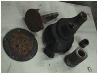
parts to make sure there are no cracks in the housing or extensive wear on shaft and bushing.
