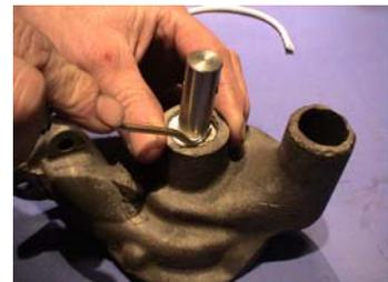
By rotating the butt joint you ensure a better seal.
