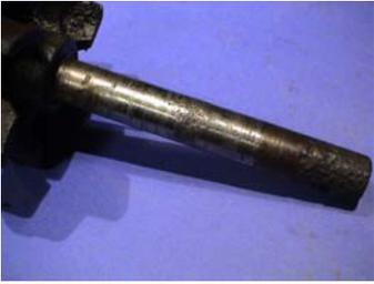
To do so, clamp the shaft into a vise with the pin facing up. Take a center punch and punch the pin that holds the impeller in place. Try to hit the middle of the pin.
