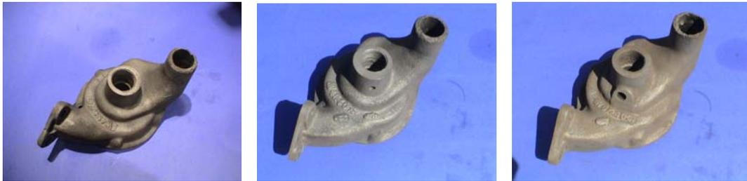
The W5 pump on the right shows a drilled and taped hole for an Almenite grease fitting or a grease pot.
