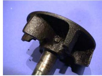
the pin is only 3/16" in diameter so do not over size the hole.
