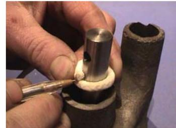
Push the strips in between the housing and the shaft without twisting the packing. You can purchase special tools for installing the packing or use a dental tool.
