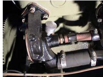
Now that you have the pump in your hand it is easier to open up the back and to remove the packing nut. With the round cover off and the packing nut gone you can push the shaft out of the housing. After cleaning the parts you have to make an inspection of the
