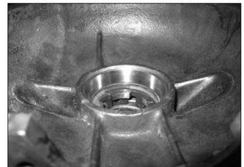
The easiest way to continue with the next step of assembly is to support the driver's side half of the axle housing in the vertical position as shown and then set the carrier unit into the bearing race. Be certain the carrier unit is positioned with the ring gear teeth facing the correct side otherwise the axles will rotate in the wrong direction with respect to the pinion gear rotation.
