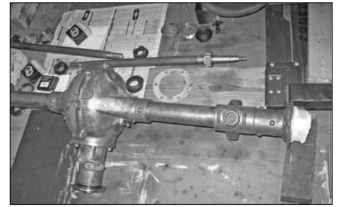
rings into the housing. Follow the adjustment procedures for the bearings to the proper axle end play and lock the adjustment rings after the brake backing plates are in place. As shown in the next photo, the differential assembly is ready to be installed on the vehicle's leaf springs and filled with the modern day gear oil. ❖
