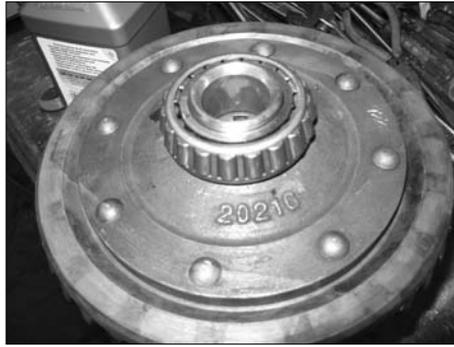
the original tapered roller bearings were no longer available and the new replacements were of a more robust design. The next photo was taken of the width modified adjustment ring and outer bearing race prior to the assembly.
