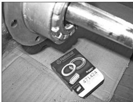
To solve this issue, I machined the inside diameter of the axle adjustment rings slightly larger where the new standard seals would press into the ring bores. The photo shows the new seal in
