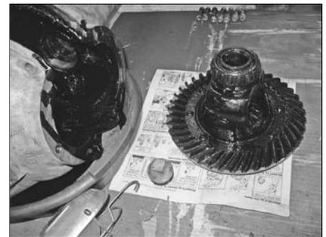
Each wheel end of the axle housing has a large threaded adjustment ring that is clamped by a locking bolt and locking pawl that couples into one of the adjustment notches on the ring. They were disassembled to allow the axles to be taken out from their respective housing sections. The photo below shows the layout of the original axle seal, adjustment nut, axle bearing outer race, and locking bolt.
